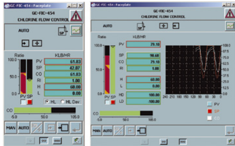
Figure 12. Control faceplate views: Normal and Extended
