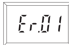
Self-diagnostic error on the integral indicator (Faulty transmitter)
